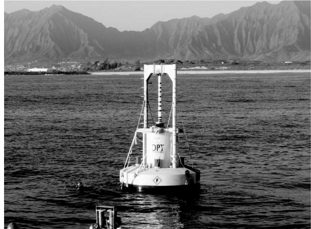
Our PowerBuoy system consists of a floating buoy-like device that is loosely moored to the seabed so that it can freely move up and down in response to the rising and falling of the waves, as well as a power take-off device, an electrical generator, a power electronics system and our control system, all of which are sealed in the unit.
