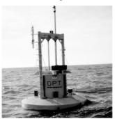
Our PowerBuoy system consists of a floating buoy-like device that is loosely moored to the seabed so that it can freely move up and down in response to the rising and falling of the waves, as well as a power take off device, an electrical generator, a power electronics system and our control system, all of which are sealed in the unit.
