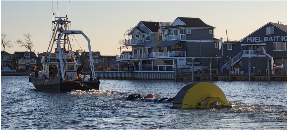
(Image: OPT MOSWEC Buoy leaving dock for deployment off New Jersey Coast)
