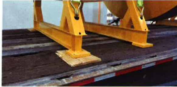
Figure 7 Shipping stand details
