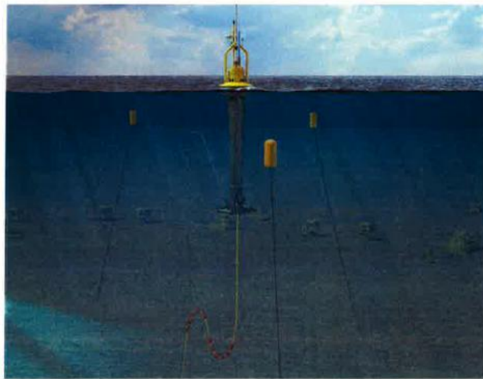
Figure 1. PB3 PowerBuoy® with 3-Point Mooring and Umbilical
