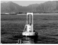
Our PowerBuoy system consists of a floating buoy-like device that is loosely moored to the seabed so that it can freely move up and down in response to the rising and falling of the waves, as well as a power take-off device, an electrical generator, a power electronics system and our control system, all of which are sealed in the unit.
