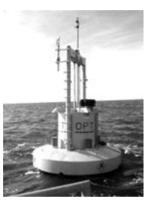
Our PowerBuoy system consists of a floating buoy-like device that is loosely moored to the seabed so that it can freely move up and down in response to the rising and falling of the waves, as well as a power take-off device, an electrical generator, a power electronics system and our control system, all of which are sealed in the unit.
